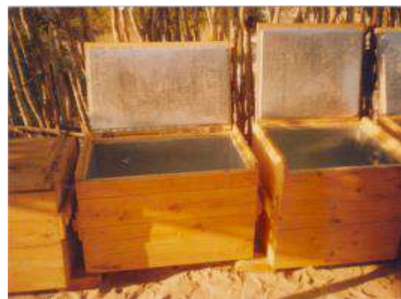
Type of cooler proposed: between the boards and galvanized flat steel, there is polystyrene. If the cover is kept closed, the ice with the product can go a week. It is experimented and used as part of a project implemented in Toliara by a UNDP/FAO project of artisanal fishing development.
